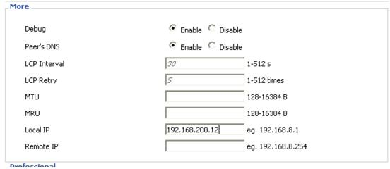
After VPN connection is built up successfully, we can reach the IP address of M2M router from center directly by IP 192.168.200.12 . So it means the network is completely satisfying the system requirement.
