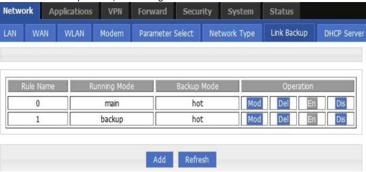
RuleO is for checking ethO, if wan link fail, the link will switch to backup link.
