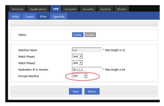
And to detect IPSec connection, and trigger it to restart when link switches, need to setup ICMP detection: Make the source interface "br0" and make the command: killall ipsec\_init
