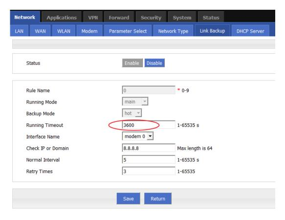
Rule1 is for checking modem, When Main link is resume available, the link will switch to main link.
